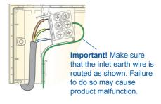
Firmly connect the conductive exert strain on the terminal
